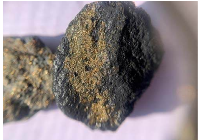
Copper mineralization (Chalcopyrite and Pyrite minerals) in Nagawanda Gold and Base metal Block
